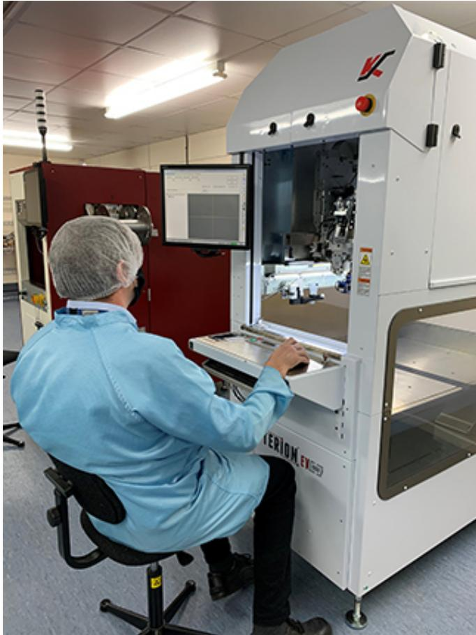
***Supplied by Inseto, CIL's new Kulicke & Soffa Asterion large diameter wire / ribbon wedge bonder will be used for the production of wide bandgap (WBG) semiconductor-based power modules and the assembly of battery packs for use in electric vehicles.***
