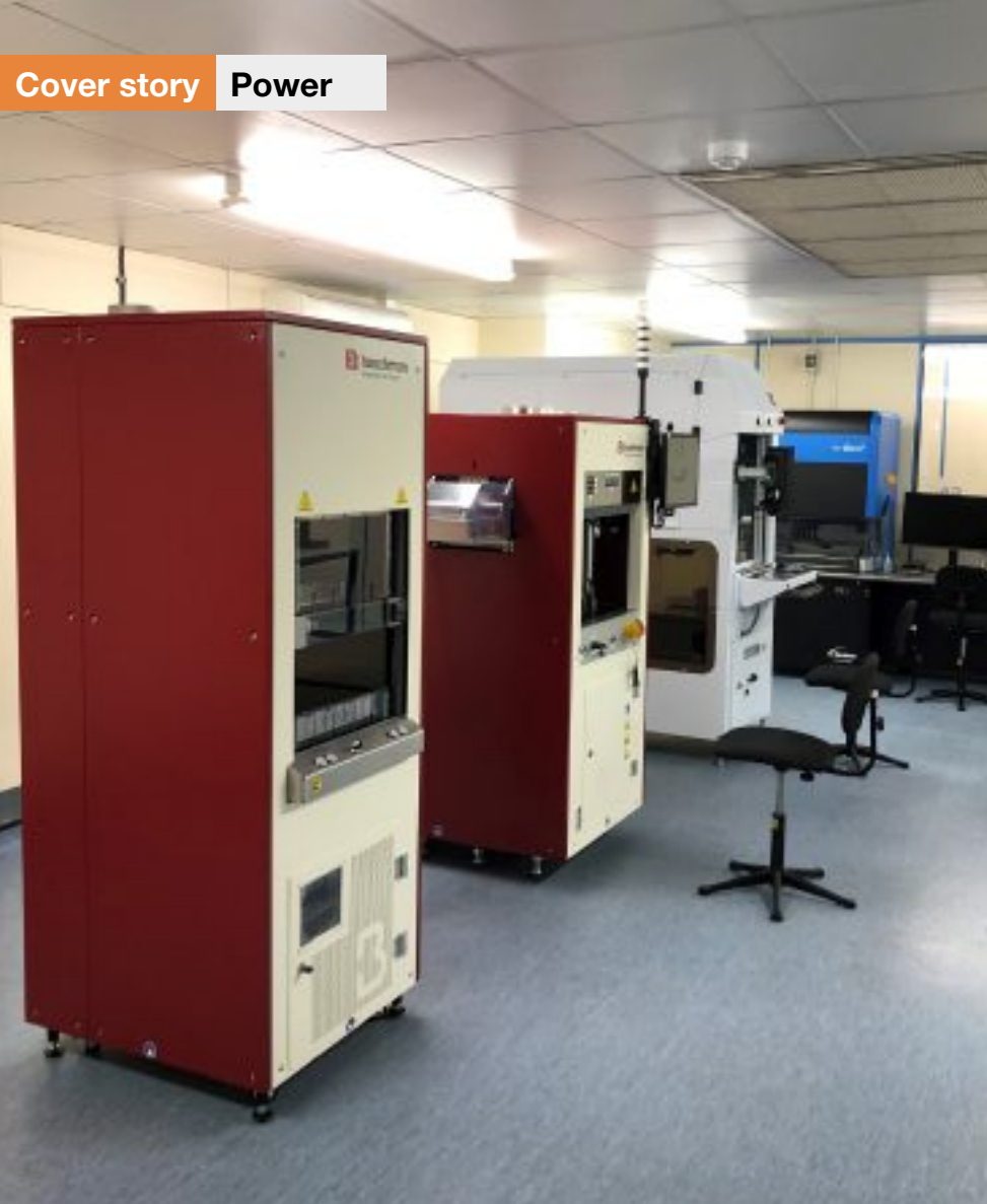
The K&S Asterion large diameter wire/ribbon wedge bonder (the white unit) is located in CIL's BEV facility and is part of a £1.6million investment to process & package WBG material die for EV power modules
