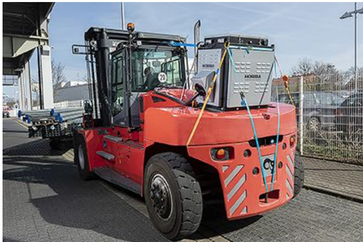
Caption: Advanced Rugged Enclosure Makes HORIBA's OBS-ONE PEMS Ideal for NRMM and HDV Harsh Environment Real World Emissions Monitoring
